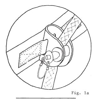
makes them overly heavy and bulky when only one channel is needed, as is the case for this ropewalker system. Devices such as pulleys mounted on carabiners let the climber hang far from the rope, making climbing less efficient. The Simmons Roller<sup>1</sup> (fig. la) overcomes these problems, since it was designed for the purpose for which it is used.
