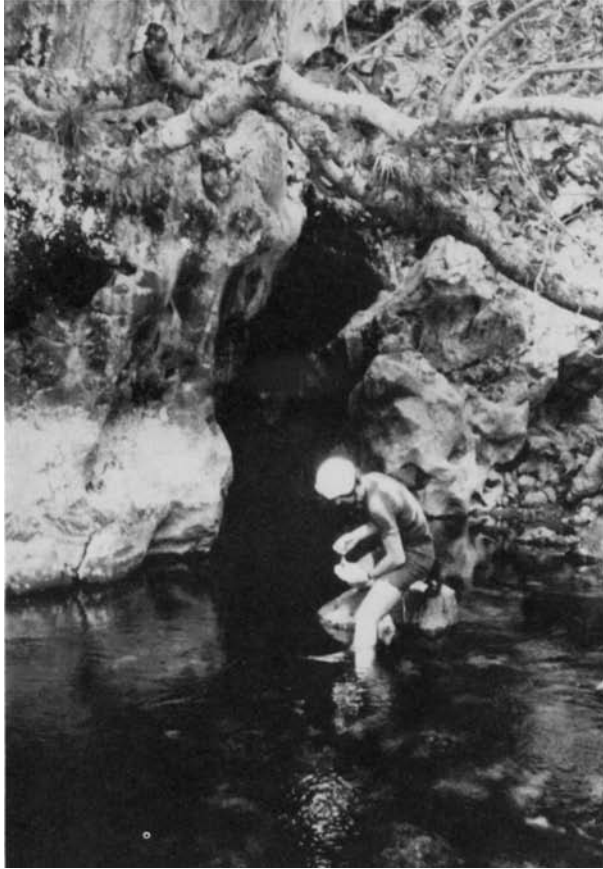
Placing activated charcoal traps at the western resurgence in the Santo Domingo canyon. (Pat Wiedeman-Stone)
