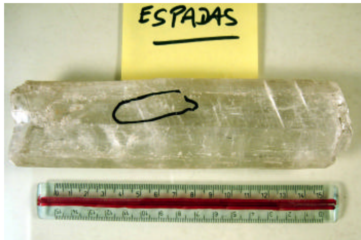
One of the crystals with large biphasic fluid inclusions
